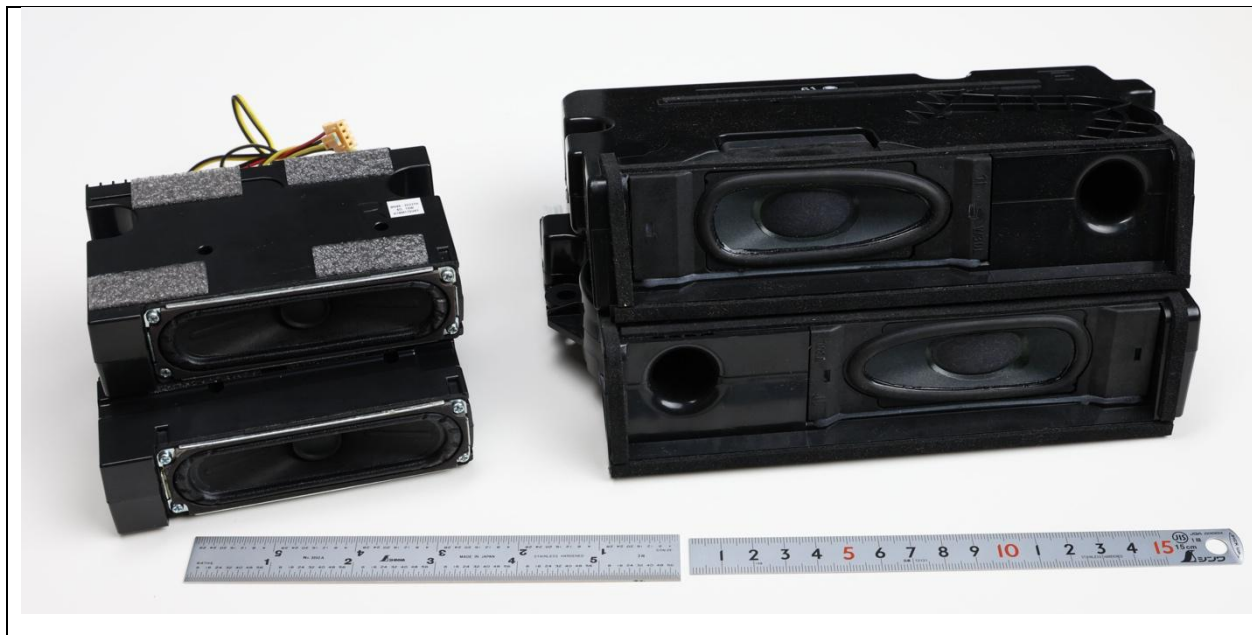
Figure 9. Speaker system of typical TV
