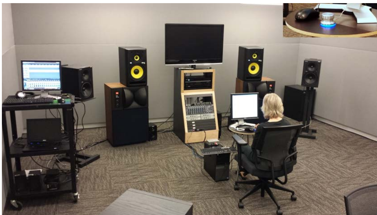
Figure 5 - Audio test room showing mid-field monitors (yellow cones) and playback volume control (inset)
