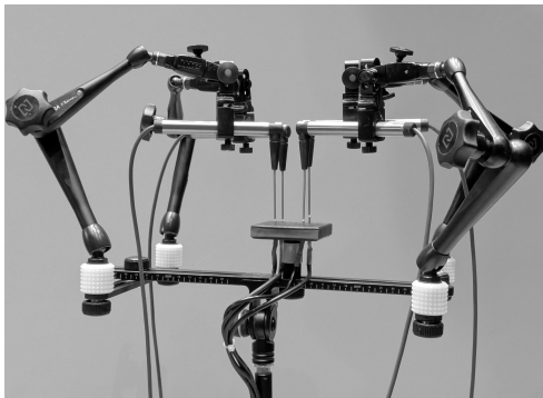
Fig. 3: View of the test jig and the custom probe array positioning for IMPro measurements.
