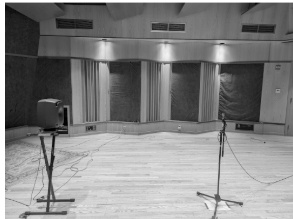
Figure 1: Impulse response acquisition setup for the RRF condition. The three fabric areas on the sidewalls were covered for the IEC condition.
