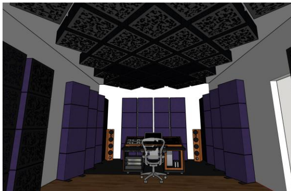
Figure 1. A design rendering of Ayan Mastering, showing Soffit Bass Traps in the front corners and dozens of Sound Blocks in freestanding configurations along the walls, and mounted on the ceiling. These are also a mixture of absorptive and binary diffusive.
