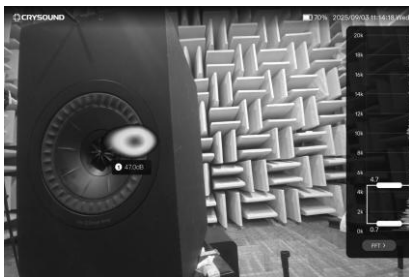
Figure 6: Beamforming on a cracked cone.
