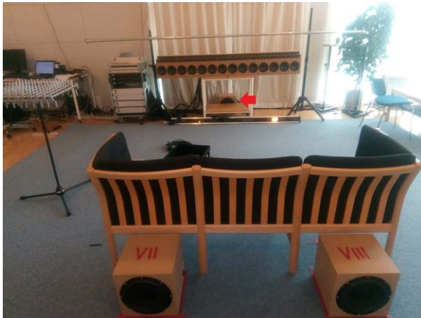
Fig. 2. The experimental setup with the domestic system placed in front of a three-person sofa. Two subwoofers are placed behind the sofa, and one subwoofer is placed beneath the domestic system (see red arrow). The other five subwoofers are placed around the sofa (see Fig. 3). A tower of amplifiers and sound cards driving the domestic system is seen to the left, and next to it is the control station with a stationary computer and laptop for running the domestic system and the experimental tests. A microphone array on a tripod (seen to the left of the sofa) was used to calibrate the system before the tests.
