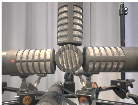
Fig. 4. Custom native B-Format Ambisonics setup.
