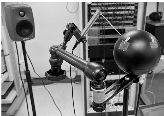
Fig. 4: Sphere microphone and probe microphone positioning for pressure frequency response measurement.
