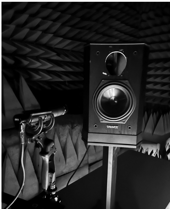
Fig. 2: Microphone and speaker in anechoic chamber
