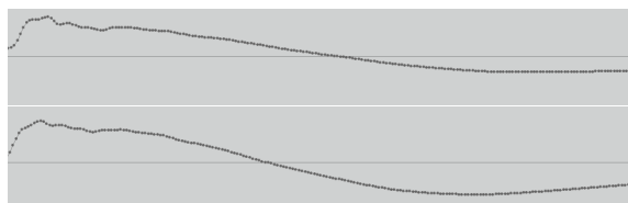
Fig. 1: Square wave half-cycle: 8 \Omega added series resistance (Top), speaker only (Bottom)
