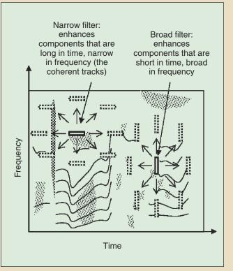
Fig. 4. Representation of Maher's 2-D filtering concept
