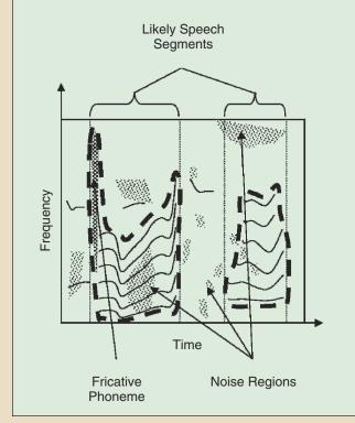
Fig. 3. Noisy speech with segments identified (Figs. 3 and 4 courtesy Maher)
