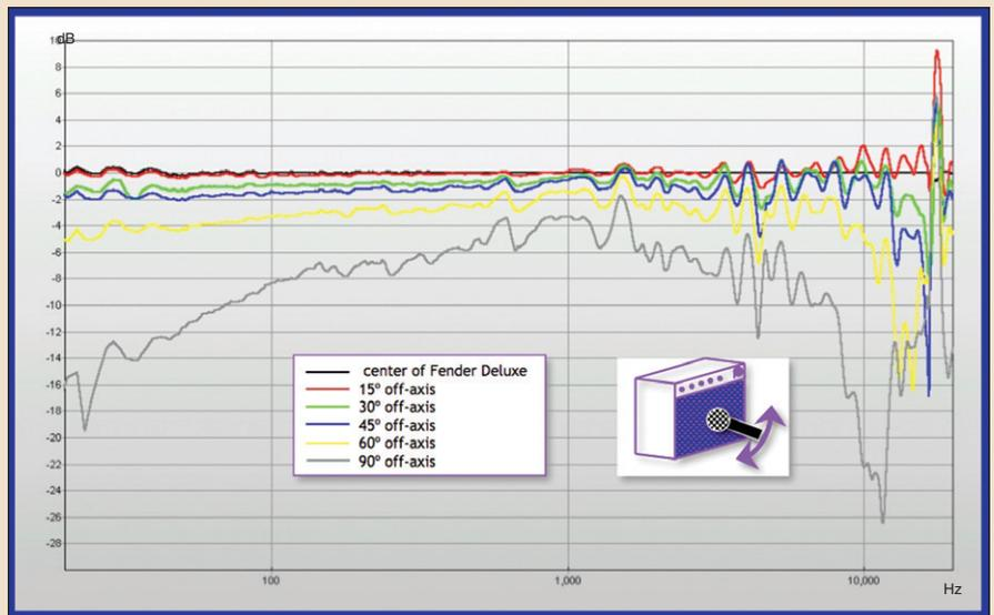
Fig. 10: Off axis microphone orientation • normalized to 0"
