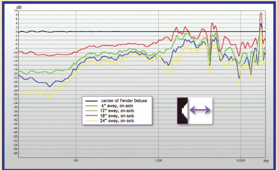
Fig. 6: Moving away from driver • normalized to 0"
