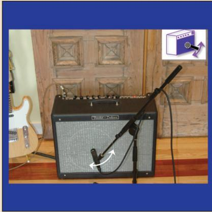
Fig. 8: Off axis orientation
